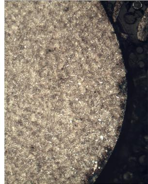
*Milling versus EDM: Numerical and experimental investigations on wear and fatigue of splined shaft-hub connections are a core topic of IMW. Since the beginning of 2017 it's possible to use our own wire EDM machine to manufacture special profile geometries. First fatigue tests with standard geometry made by wire EDM and milling, showed a significant loss of fatigue resistance for the parts made by EDM.*
